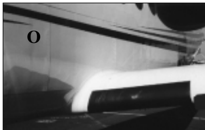
The multi-segmented, displaced hinge flaps and leading edge slats on the C-17 give a tremendous increase in chord and camber.
